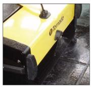
**Solution Atomization** Cleaning solution is atomized into a fine mist and dispersed through the cylindrical brushes, so less moisture is consumed during the hard floor or carpet cleaning process.
